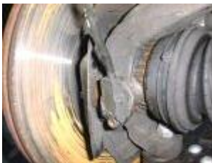
ABS road speed sensor sitting beside the crown wheel.
