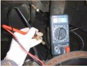
Measure the resistance of the road speed sensor.
