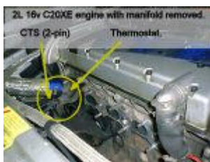
2L 16v C20XE engine with manifold removed. CTS (2-pin) Thermostat. CTS located on 2L 16v engine.
