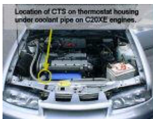
Location of CTS on thermostat housing under coolant pipe on C20XE engines. CTS located on 2L 8v engine.
