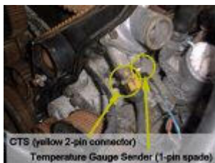
CTS (yellow 2-pin connector) Temperature Gauge Sender (1-pin spade) CTS located on 2L 16v Ecotec engine.
